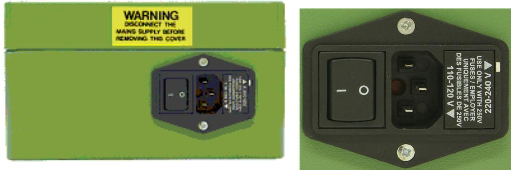
The picture shows the voltage selection set to 240v ac. To change to 110v ac remove the fuse holder and re-insert with the 110v arrow pointing towards the white line.
